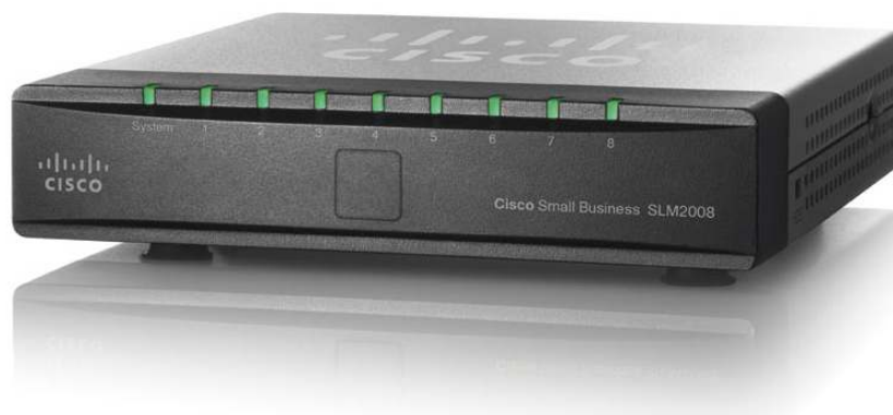
Figure 1. Cisco SLM2008 8-Port Gigabit Smart Switch
